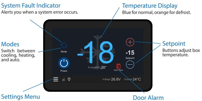
Adjust brightness, temp unit, and view serial number.
